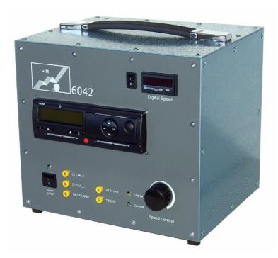
This is a small and compact unit to drive a digital tachograph via a motor nearly in order to simulate driving a vehicle. An ideal tool for those who need to test and prove software programmes when compiling software programmes in
